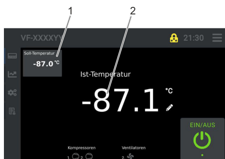
Fig. 104: Cooling chamber temperature set point icon
